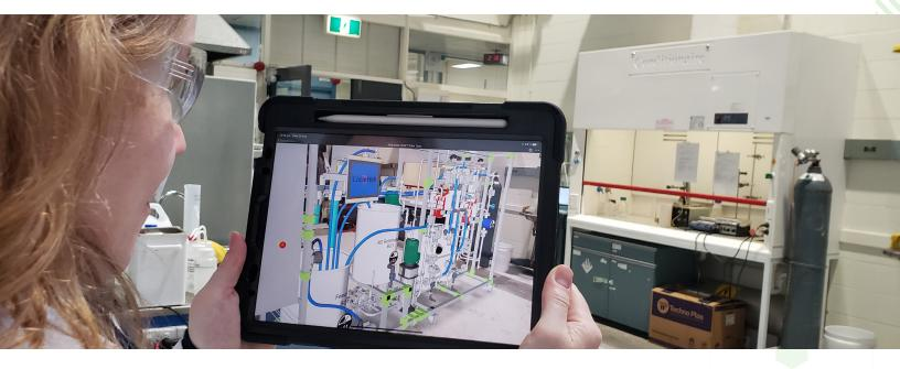
Those experiences will be connected to the Thingworx IoT/digital twin platform and Ansys simulations to create an AR-based Human Machine Interface (HMI) to expand on-site accessibility to the physical equipment via remote and simultaneous access to the digital twin.
