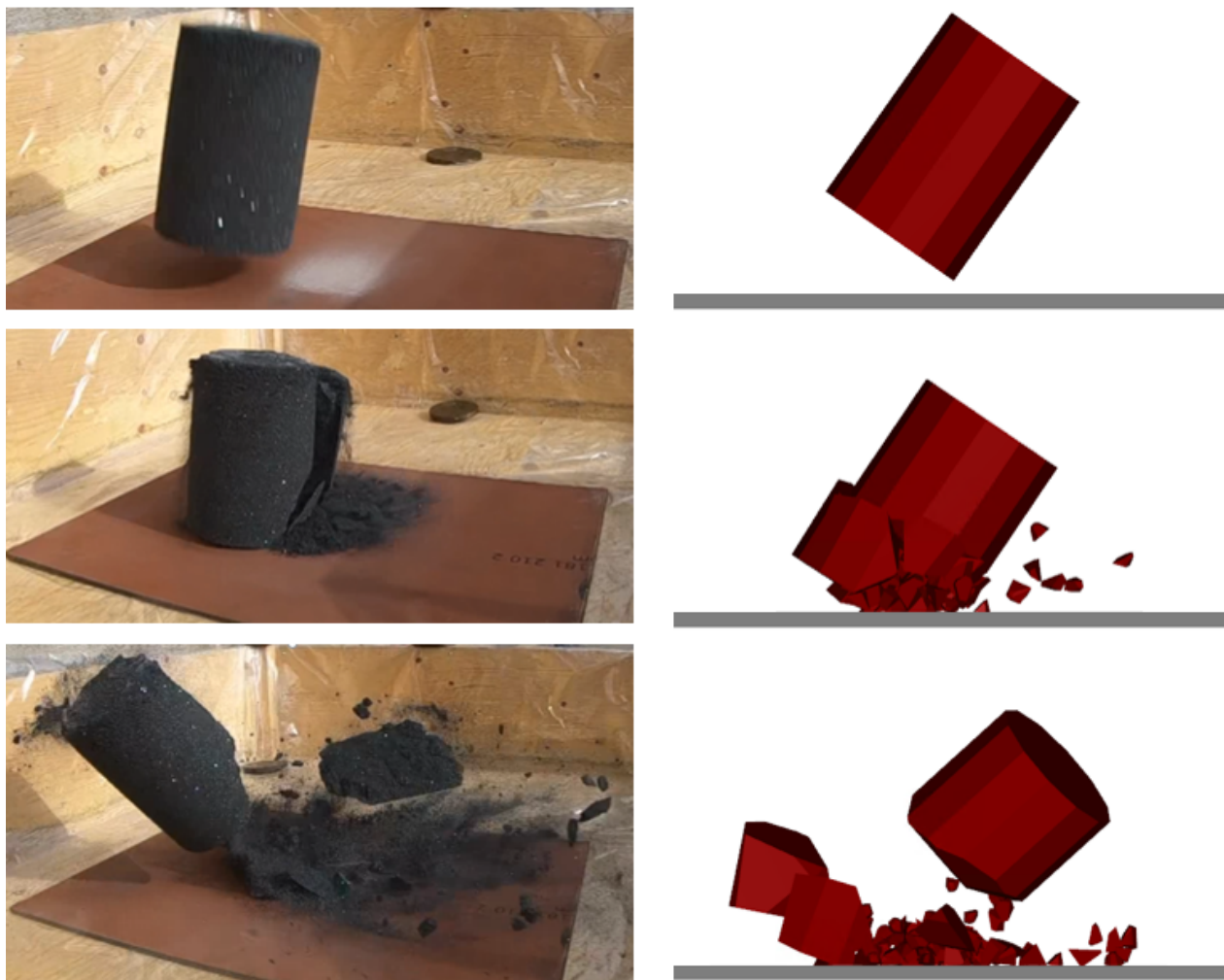
Conversion of breakage from the laboratory to DEM "digital twin".
