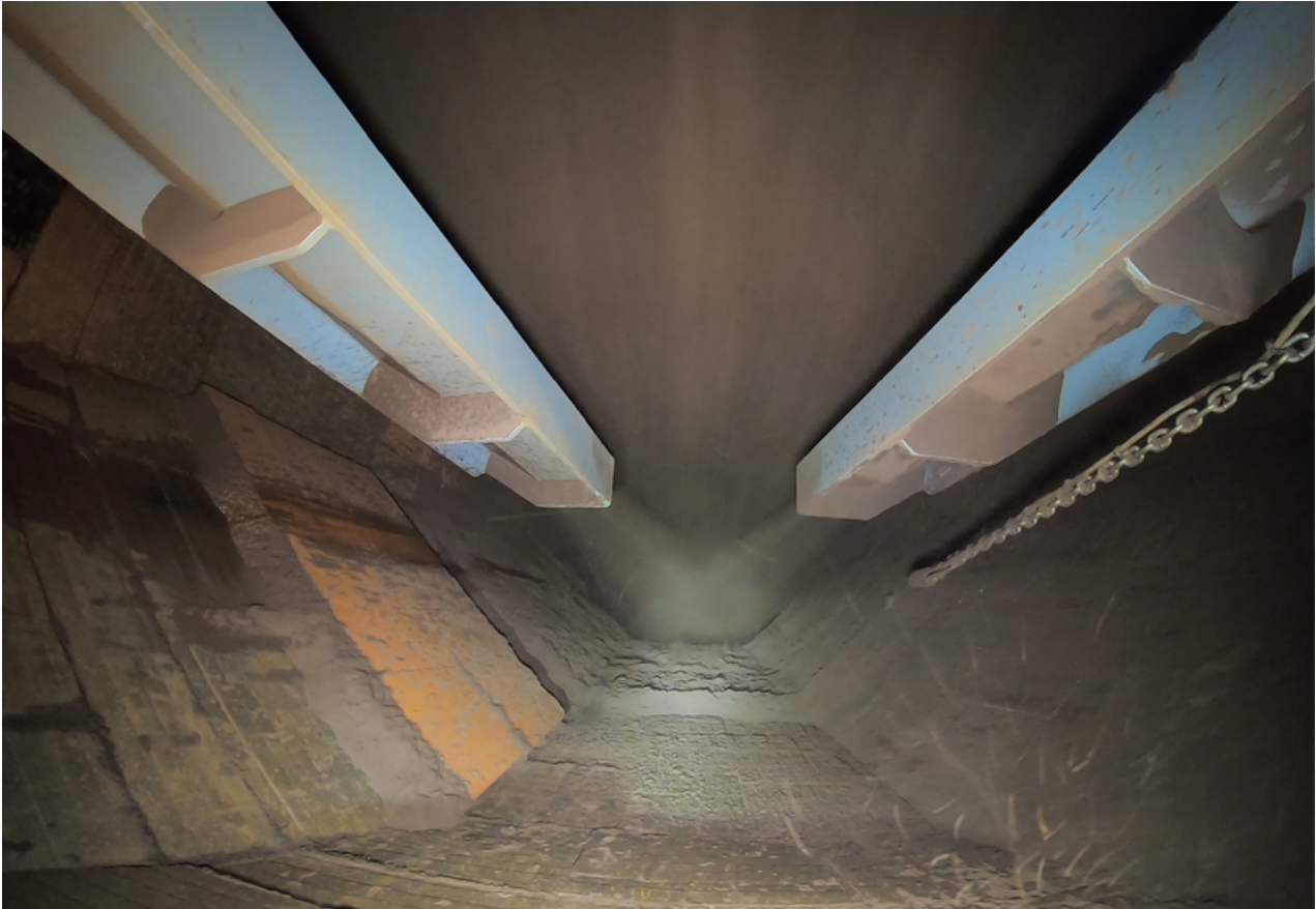
Figure 6: Ore discharge from wings, central feed presentation to lower chute.
